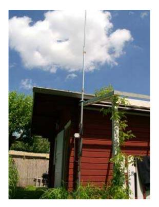
The aluminum pipes plug together telescope-like. The 4 thinner bars of the upper 4000mm are pre-drilled and with 2 tapping screws each per junction point bolted.
