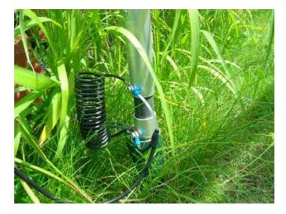
At the feed, which takes place with 50 ohms of coaxial cables, is a coil with 17 turns on 20mm with an approximate length of 140mm. It derives static loadings. The wire should be rigid because of stability. Copper wire with 1 to 2mm is OK. At the lower part of the feed the radial net is attached. Here is to be paid attention to particularly good contacting with a broad ground strap.
