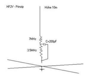
The condenser sits with a contact directly at the coil. The other contact short circuits the lower part of the coil with an aluminum handle during excitation with 7MHz. During excitation with 3.5 MHz the condenser is high impedance, the jumper is ineffective.
